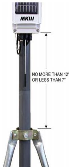
2. Rotate the assembly until the solar panel faces TRUE SOUTH. Secure the support tube to prevent rotation.
