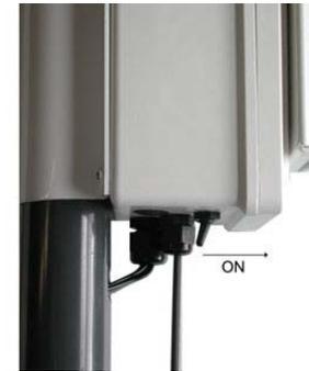
3. Turn the system on by pulling switch forwards towards the front of the unit. The switch will click into position. The system is now transmitting.
