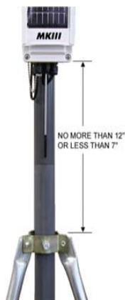
1. Mount the support tube as indicated above. Insert the necked down end into the **MKIII** sensor assembly, until it bottoms with the retaining screw in the slot. Tighten the screw.
